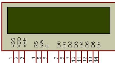
The most commonly used Character based LCDs are based on Hitachi's HD44780 controller or other which are compatible with HD44580. In this tutorial, we will discuss about character based LCDs, their interfacing with various microcontrollers, various interfaces (8-bit/4-bit), programming, special stuff and tricks you can do with these simple looking
