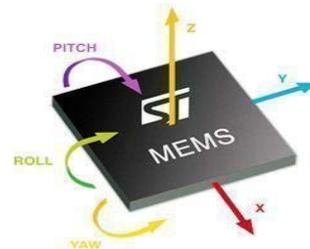
While electronic circuits are inherently solid and compact structures, MEMS have holes, cavity, channels, cantilevers, membranes, etc, and, in some way, imitate ‘mechanical’ parts.
